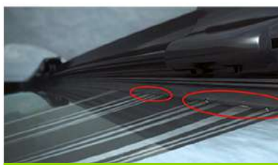
Cracked blade Essuie-glace fissuré
